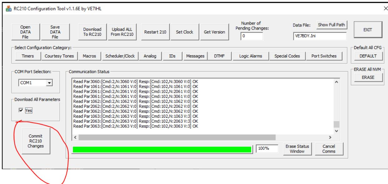
Always use the **Save DATA File** button after making any changes. When restarting the RC210 configuration tool, use the **Open DATA File** button to read in your previously saved configuration data.
