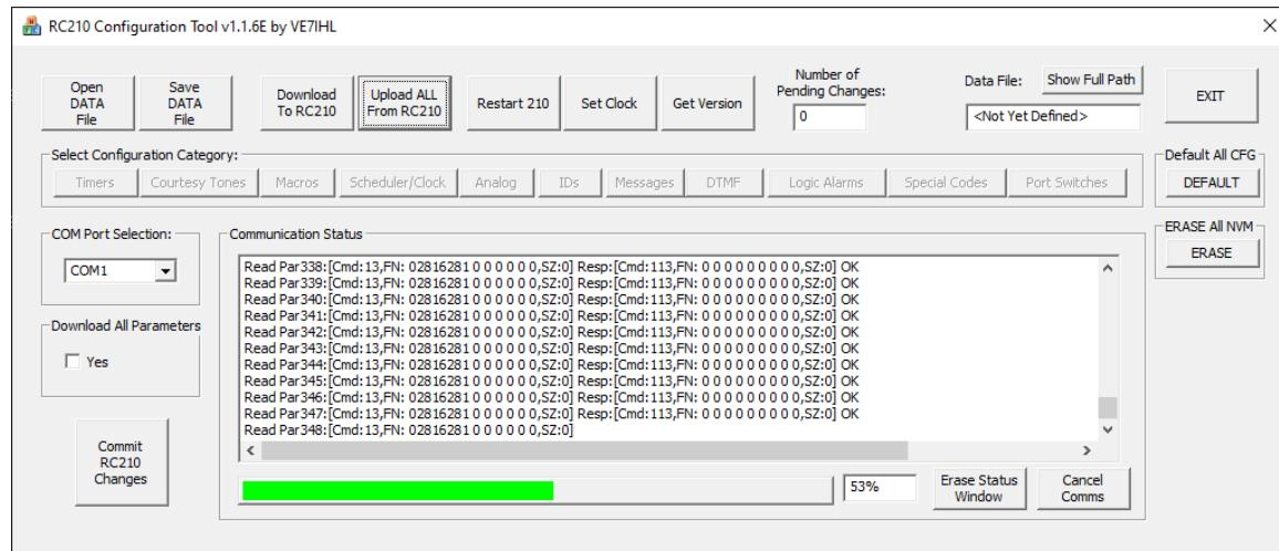
Wait for all the configuration parameters to be read from the RC210 board, (Progress box will go to 100%).
