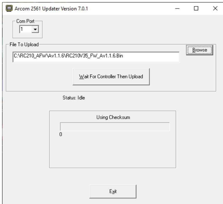
Use the **Browse** button to locate the alternate RC210 firmware .bin file:
