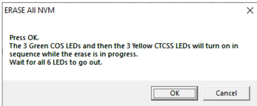
Press OK. Wait for all 6 LEDs to go out. Proceed to the next section to write in factory default configuration parameters.
