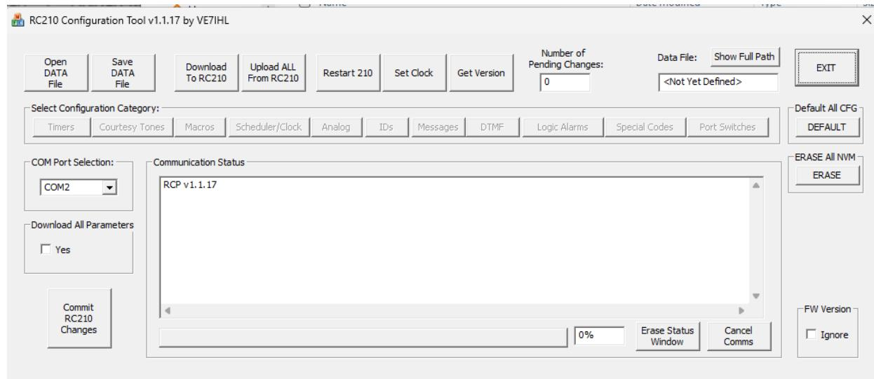
To confirm that serial communications are setup correctly between the RC210 Configuration tool and the RC210 serial port, press the **Get Version** button. It should return the current alternate RC210 firmware version number:
