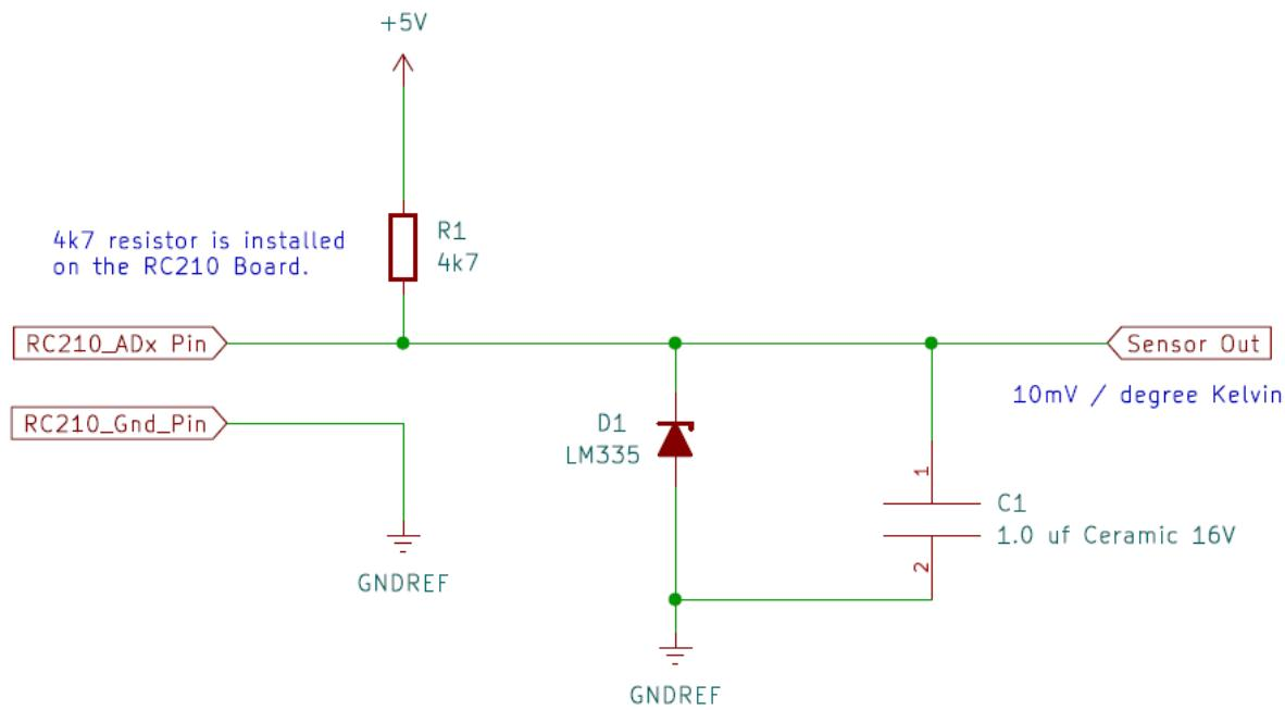
For the analog temperature sensor calibration to work, YOU MUST remove the Zener protection diode on the analog input pin. This will be diodes: D15 for DB25 input pin 1, or D13 for DB25 input pin 2. If using one of the other DB25 input pins, then the associated diode(s) to remove are: D4, D5, D7, D8, D10, and/or D11. You can easily “clip” one leg of the diode and leave the diode installed in the pcb to accomplish this.
