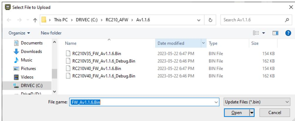
Click Open. Then click the **Wait For Controller Then Upload** button, and ensure the upload proceeds without errors.
